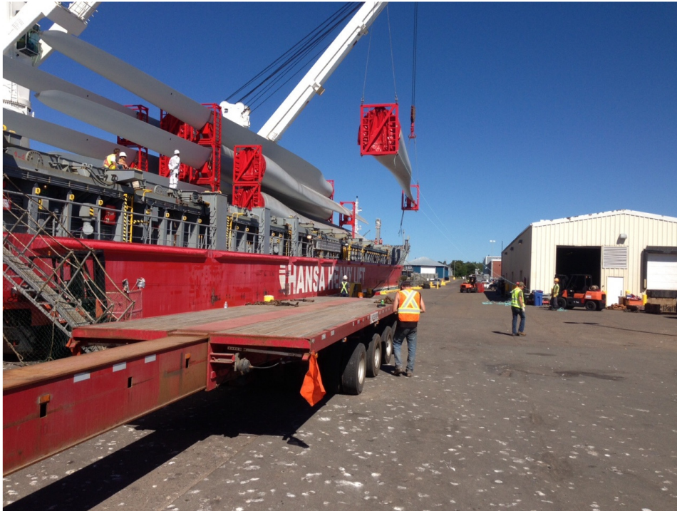
Landing 57.3 metre blade on trailer at Berth 1 - September 2013
