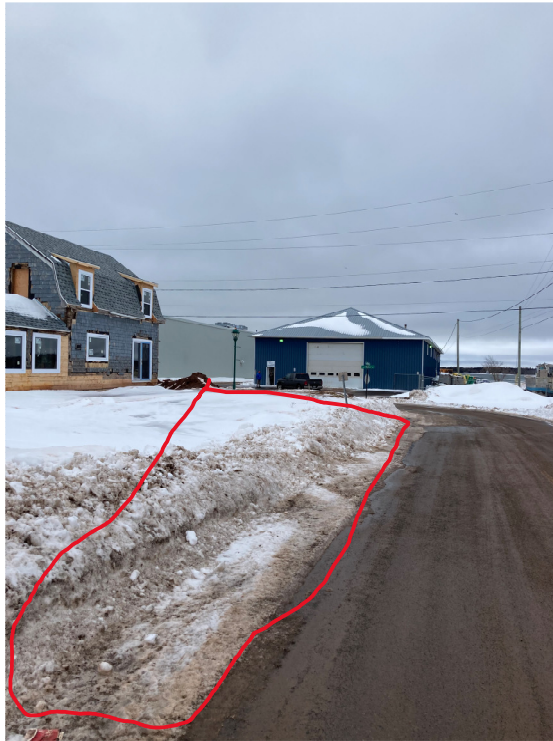
View of house and entrance to Berth 1 from West Street. The red highlight indicates area of homeowner's front lawn that would have to be excavated and replaced to accommodate trucks and blade trailers
